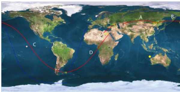
Figure 3: ISS ground track segments A-E chosen for filming purposes to most closely match the ground track and time of day of Vostok-1(see Fig. 1).
